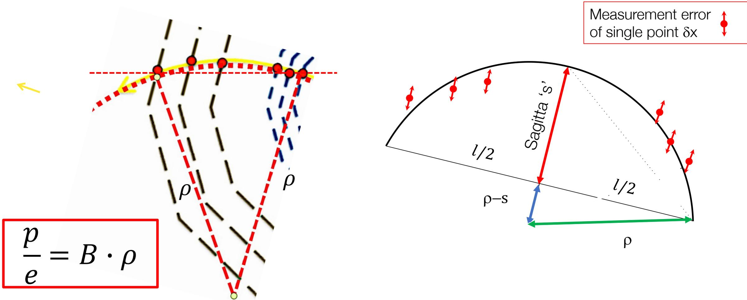
Momentum is determined by measuring the radius of curvature in magnetic field  $p \propto \rho$ .
