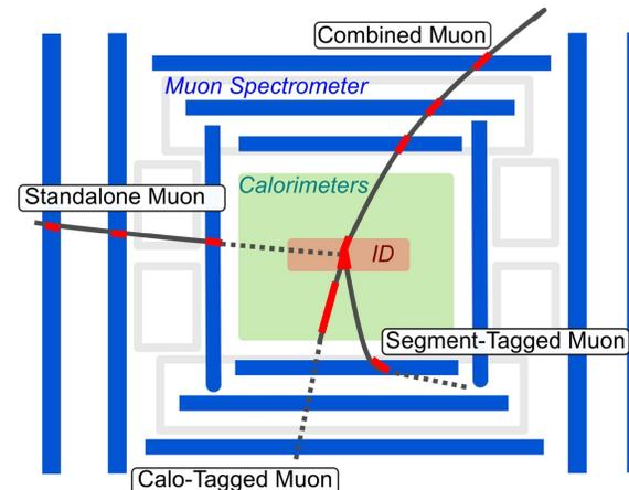
Note: calorimeters filter ALL particles but Muons !
