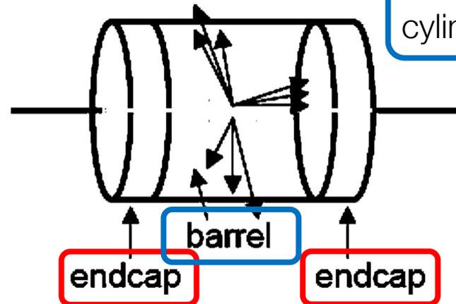
the barrel (large angle / large  $p_T$  / large  $\eta$ ) cylindrical and co-axial with the beam axis
