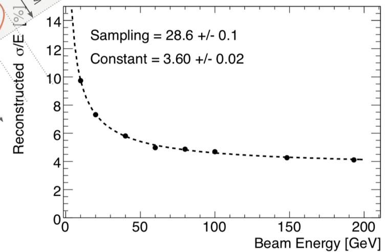
The signal of a shower is linear with energy, the resolution decreases with energy
